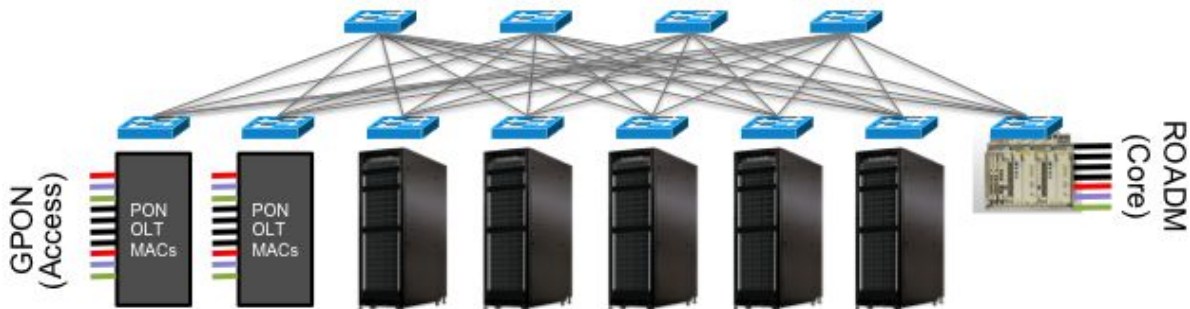
Figure 1. Target hardware built from commodity servers, I/O Blades, and switches.
